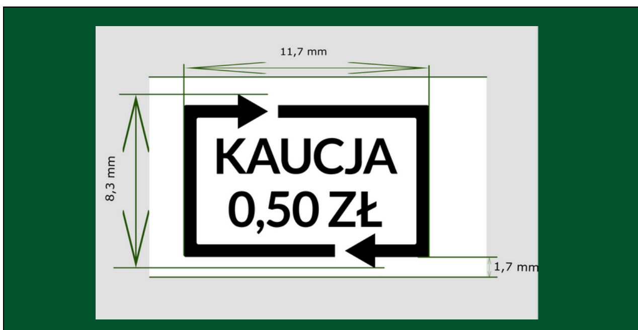
Size of the protective field for the minimum sized marking for the deposit system
